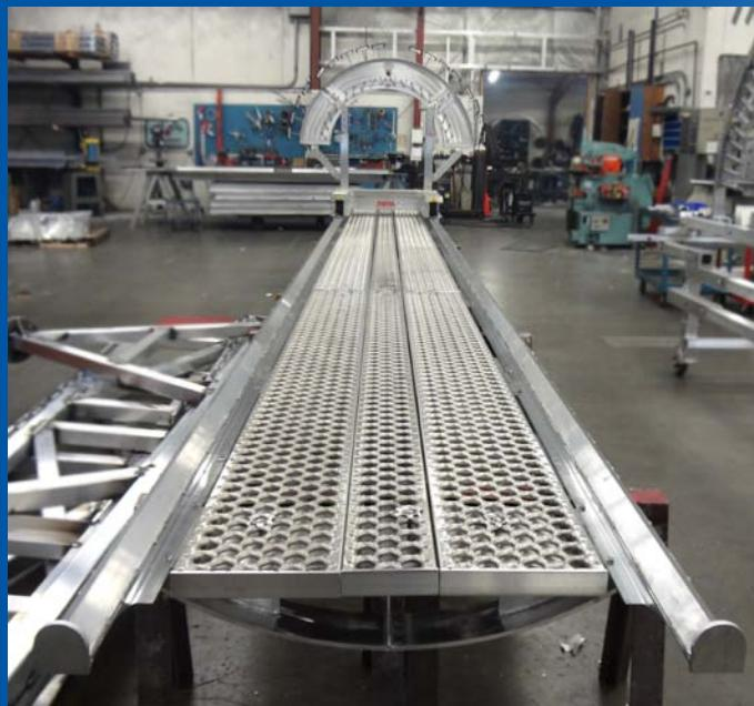
Designed and fabricated out of 6061-T6 aircraft aluminum with custom Aluminum Perf-O-Grip Planking and a 2,722 kg (6,000 kg) net capacity aluminum frame with rails to support trolley
