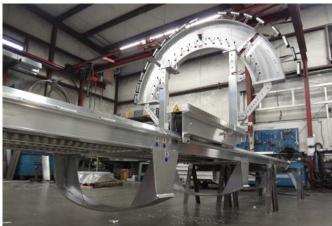
Cylinder bumpers articulate to allow full contact with the refractory. **3 Way Master Valve** allows for independent operation or all cylinders simultaneously.
