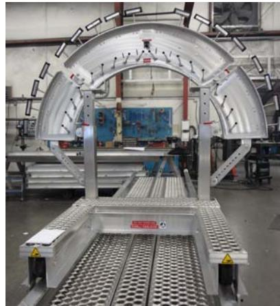
Custom made flex arch with flexible hinge connections to allow arch wings to adjust toward and away from kiln wall. Arch stabilizer post to adjust proper distance of arch from shell
