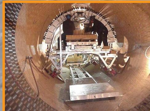
Lightweight, aluminum, modular system for transporting full pallets of brick into the kiln.
