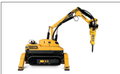
Hydraulic breaker in images: BHB 155 Load and stability diagram available on request
