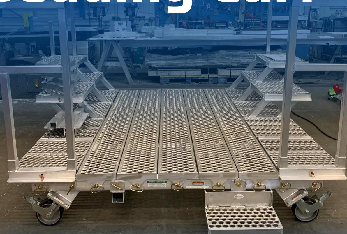
**Speed up bedding out larger kilns while providing a safe, ergonomic working deck with stairs for higher brick placement.**
