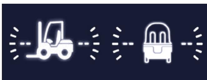
When the forklift is working on an inclined road surface, the tilt is sensed in the front, rear, and left and right directions of the equipment. A warning is given to the operator if the sensing value exceeds the preset stability range.
