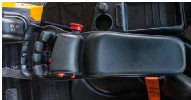
The response time (within 0.1 s) and fine-tuning capability of fingertip are improved, thanks to the built-in Dither control and controller current feedback systems, and its control is adaptable to the temperature of the environment.
