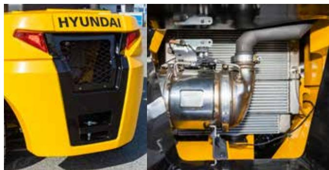
To eliminate the inconvenience of removing the counterweight to inspect the aftertreatment device inside the weight, the opening of the counterweight has been expanded to the maximum extent possible.
