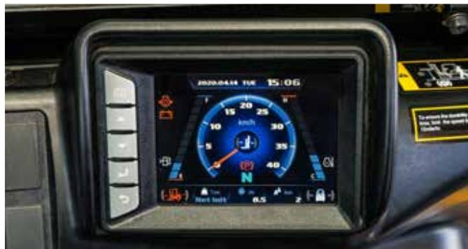
In the new cluster, the size and characteristics of the symbols have been adjusted for better visibility of driving information and safety warnings, and MCU functions are integrated to simplify parts.
