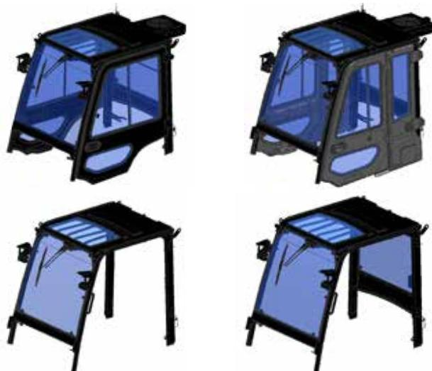
From cabin with air conditioning and heater (1Door / 2Door) to partial cabin(Front&Top, Front&Top&Rear). Various cabin options are available.
