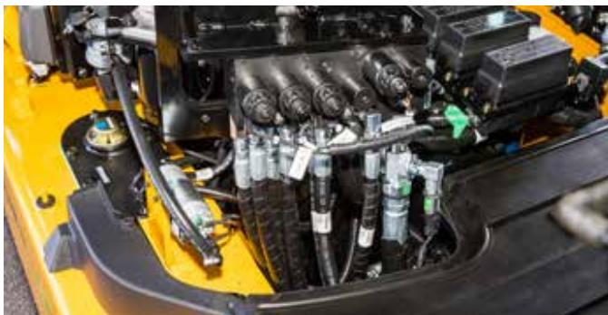
The load-sensing MCV has a very low internal leakage, resulting in a dramatic reduction of the amount of natural settlement (change in position due to its own weight) of the lift and tilt lines. Along with this feature, the Lift Emergency Lowering Screw and a Descending Speed Adjustable Regulator of the MCV reduce the maintenance frequency and downtime.
