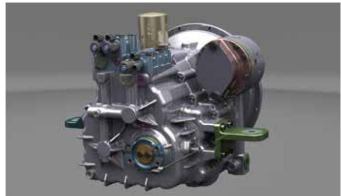
HDX's transmission and drive axle transmission, which have improved durability and practicality, increased clutch pack power transmission capability by 25% and T/M oil quantity, considering high-load working conditions. The reverse gear with a low frequency of use is made into one gear, and to the forward gear consisting of two steps is applied an automatic transmission system for increased practicality and convenience.
