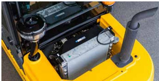
The subhood of the toolless-type radiator, which is located on the top of the main hood and the detachable counterweight, reduces downtime when inspecting and replenishing the coolant.
