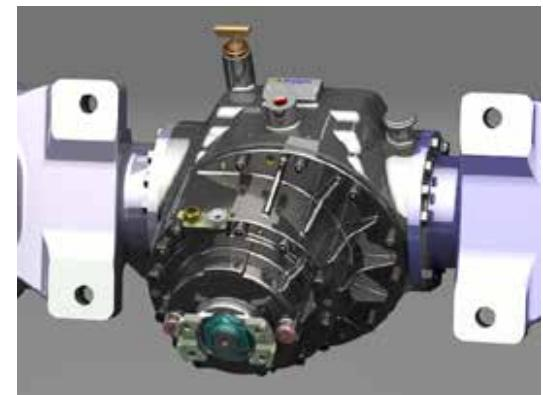
The negative-type auto parking brake operates automatically when power is cut off in order to prevent safety accidents caused by human error, like not operating the parking brake lever, and backslicing is prevented upon restarting on a slide with the Hill Start Assist Control (HAC).
