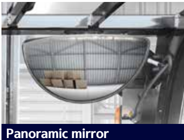
Panoramic mirror The panoramic mirror expands the driver's view when backing up.
