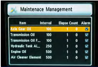
Maintenance management Replacement cycle of consumable items can be checked on the monitor, thus preventing performance deterioration of major functional parts due to failure to notice deterioration.
