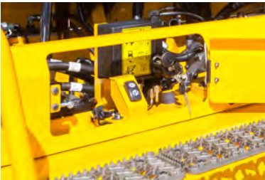
Automatic tilting system The cabin tilting system allows the operator to tilt the cabin with a single switch up to 54 degrees, thus enabling easy maintenance of functional devices located under the driver seat.
