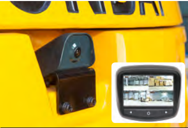
Rear view camera A rear view camera and monitor are linked to the reverse gear, ensuring safer rear work environment.
