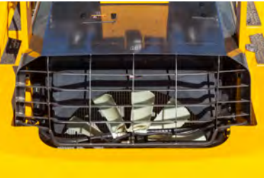
Up-to-date cooling system Variable speed and remote controlled fans reduce fuel consumption and noise, while the aluminum cooler improves durability and heat output.
