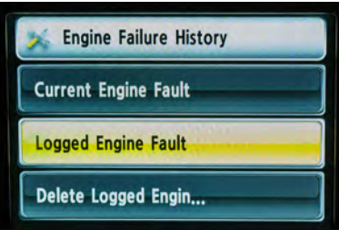
Engine fault diagnosis Details of engine fault diagnosed by the engine control unit (ECU) can be checked on the cluster.
