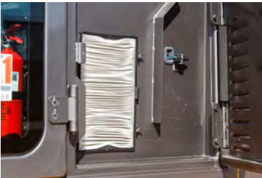
Cabin air cleaner filter The air cleaner filter blocks external dust and noise from the cabin, and continuously supplies clean air indoor to maintain fresh air in the driving space.
