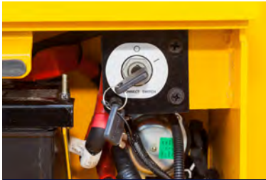
Battery master switch Damage is prevented during inspection/maintenance of electronic units, and battery discharge.
