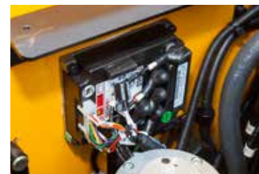
Reliable MOSFET type controller
