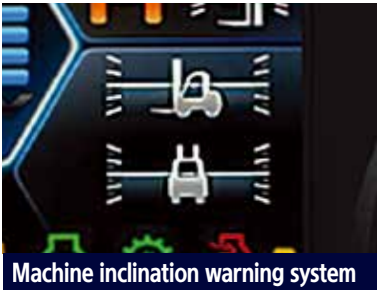
Machine inclination warning system
