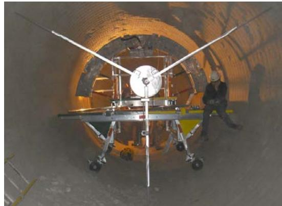
The laser target is a three armed self centering assembly that accurately centers the target on the centerline of the kiln. Please refer to separate set up directions provided with the unit. For burner tube adjustment using the laser slighter, the target assembly should be placed 25-30 yards/meters up the kiln from the laser beam source.
