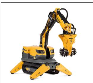
Hydraulic breaker in images: BHB 105. Drum cutter in image: BDC 40.
